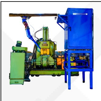
Kneader Equipped with Auto Dispensing of Carbon, Filler and Oil
